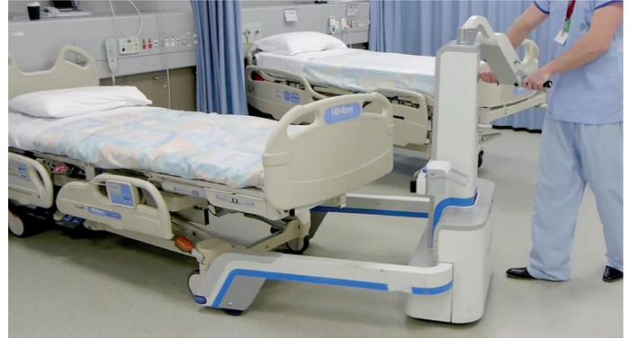
The Gzunda GZS hospital bed mover allows one person to effortlessly move heavy hospital beds. The motorised unit operates equally well with or without a patient, simplifying the task of moving beds or patients between wards, departments, or to and from theatre, allowing the driver to focus on the needs of the patient during transport.
