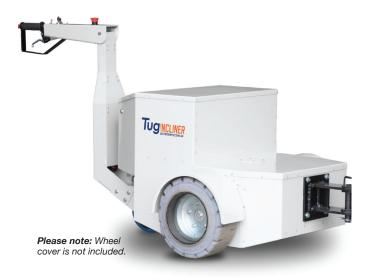
The Tug Incliner pedestrian operated electric tug has been designed to tow on slopes or ramps, and is capable of towing up to 1 tonne on a 10 degree ramp, or up to 500 kg up a 14 degree (4:1) incline with ease
