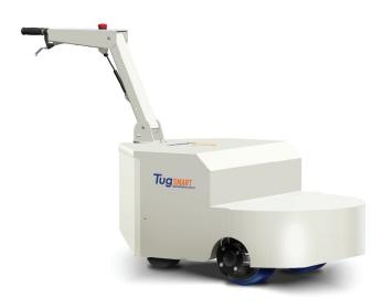
The all new Tug Smart pedestrian operated electric tug is the perfect work horse for moving very heavy loads. It is able to tow up to 6 tonnes on flat ground, up to 1 tonne on an 8° incline, or up to 500 kg on a 14° incline with ease.
