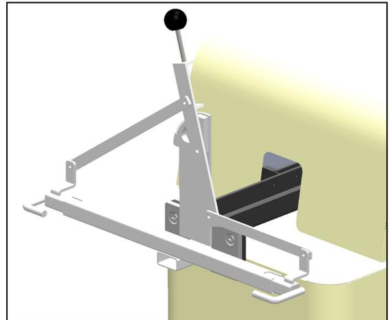
To disengage, release the locking pin and open the hooks out.
